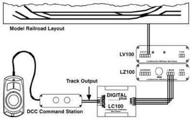
Figure 1 Connecting the LC100 to a ROCO "Digital is Cool" or LGB "Multi Train Control" DCC System
