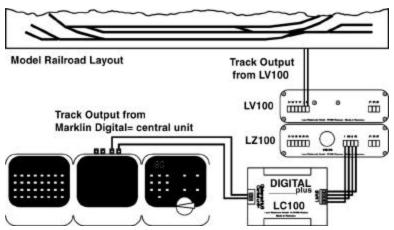
Figure 2 Connecting the Arnold or Marklin Digital= system to the LC100
